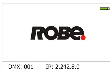
The green icon at the top right corner of the screen indicates the level of the display battery charging. If the whole icon is green, the battery is fully charged while the red icon indicates exhausted battery. The battery charges during fixture operation, its charging lasts cca 6 hours.
