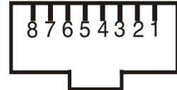
Patch cables that connect fixtures to the hubs or LAN sockets are wired 1:1, that is, pins with the same numbers are connected together:
